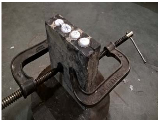
Fig. 2 AL7175- Sr Alloy poured into the Mould Cavity
